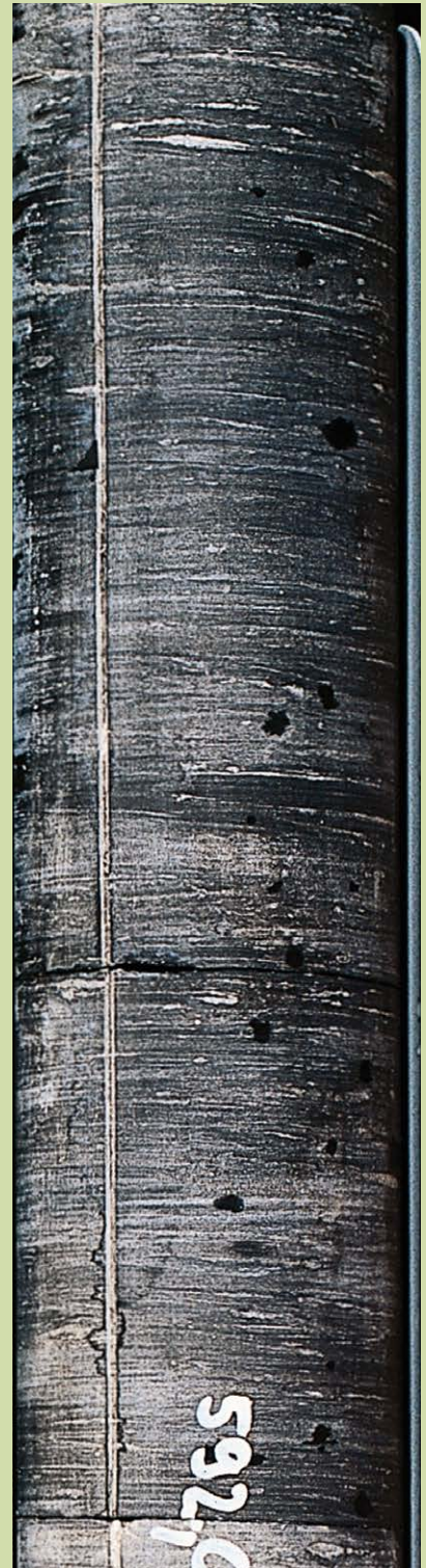
Figure 2 – Opalinus Clay of the Benken borehole in Northern Switzerland (core diameter: 10 cm; depth: from 591.6 to 592.0 meters) (source: Nagra).
