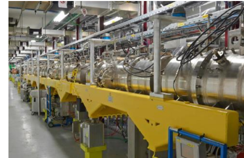
CCDTL: coupled cell DTL
