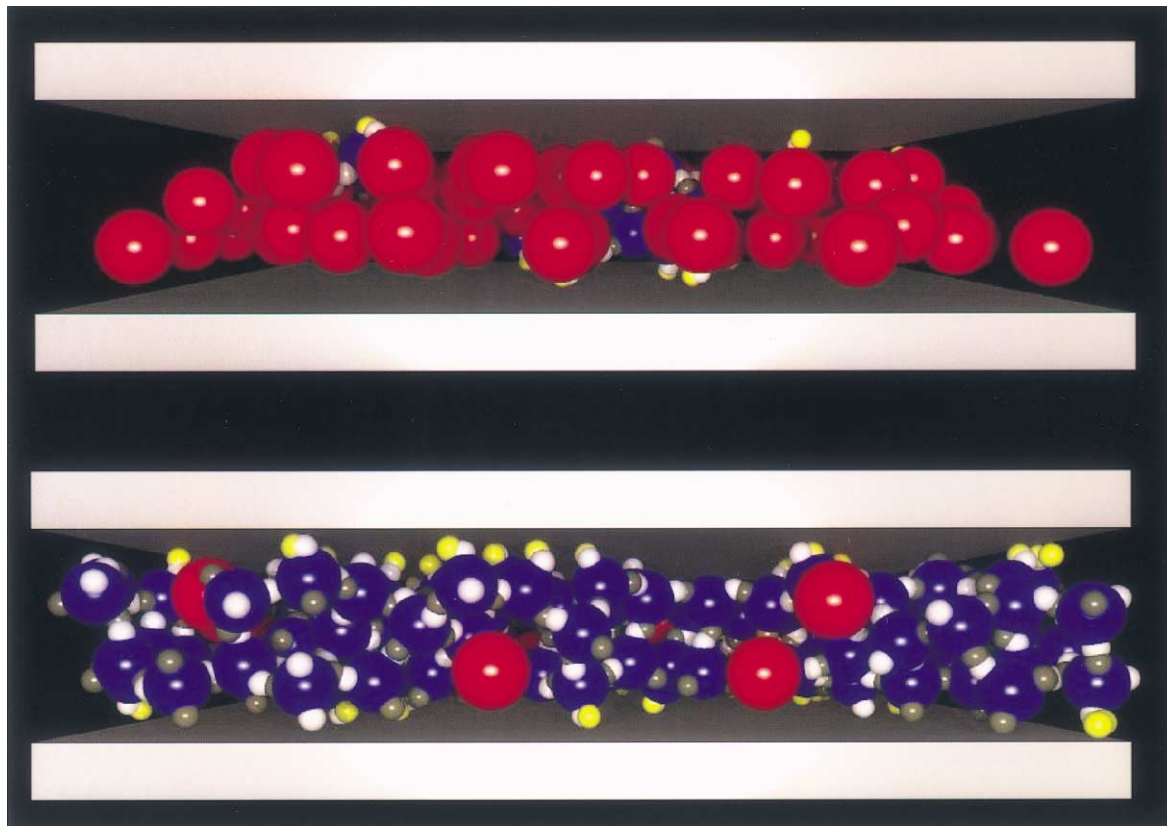
Fig. 22. Snapshots of equilibrium configurations for the adsorption of methane (red spheres) and water (blue spheres) in a pore width H = 1 nm with site densities n = 0.5 sites \text{nm}^{-2} (top) and n = 1.75 sites \text{nm}^{-2} (bottom) at 300 K. Yellow spheres represent activated sites on the surface of the pore; white and green spheres are the hydrogen and lone pair electron square well sites on the water molecules, respectively. Reprinted with permission from Ref. [131] copyright 2000, American Chemical Society.
